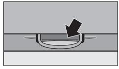
Also clean the small drip tray in the lower part of the inside of the front of the machine thoroughly.
